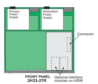
Figure C-3 Fast Ethernet Interface Module Connector Location
